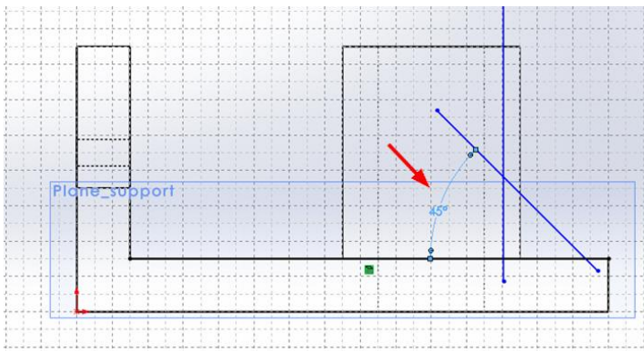
Figure 56. Use the Smart Dimension tool to apply a 45 degree angle between the inclined line and the horizontal top edge line of the bottom plate.
