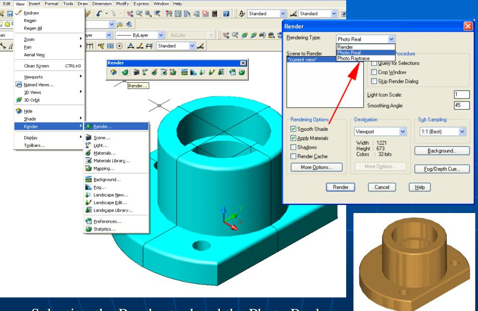
Selecting the Render tool and the Photo Real option; clicking the Render button to see the rendered model in the Model space.
