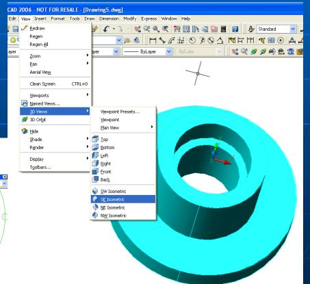
Using 3D Orbit and SE Isometric tools to view the 3D model
