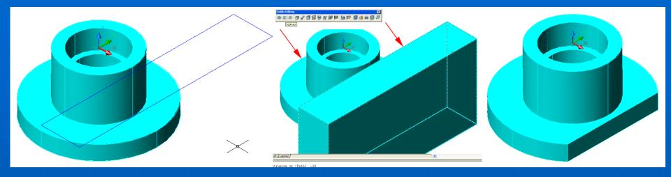
Creating the profile (left) and the prism (center, Extrude) to cut a straight edge from the base (Subtract)
