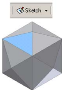
Figure 8B-2A: Selecting one of the triangular surfaces to start the Construction sketch.
