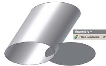
Figure 1E-5K: Placing another occurrence of the top piece, to be used as the base piece.
