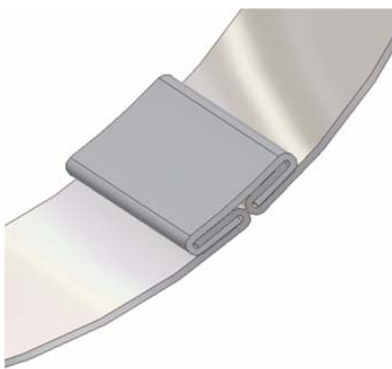
Figure 10B-3: The locking seam.
