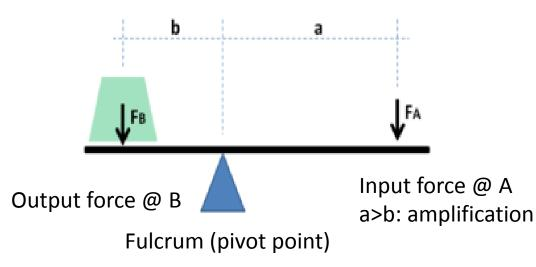
**Pivoting:** Points farther from this pivot move faster than points closer. Same power into and out of the lever
